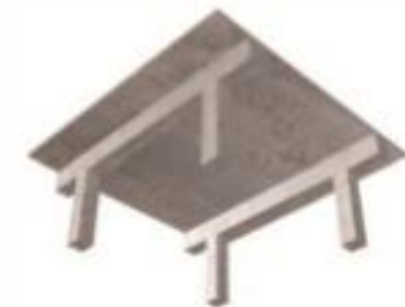
Solid slab with narrow beam
