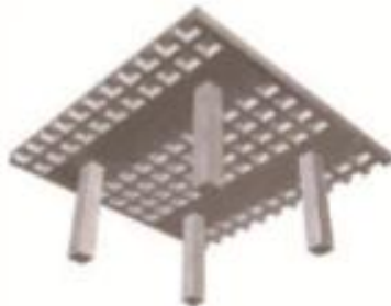
Waffle slab with band beam
