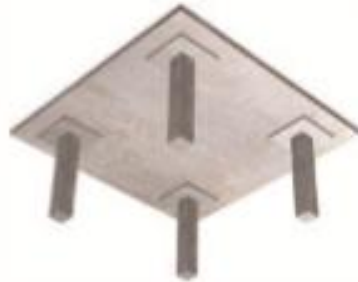
Solid flat slab with drop panels
