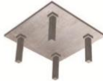
Solid flat slab with drop caps
